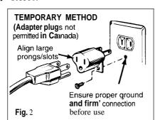
Caution: Attaching the adapter ground terminal to the wall receptacle cover screw does not ground the appliance unless the cover screw is metal, and not insulated, and the wall receptacle is grounded through the house wiring. You should have the circuit checked by a qualified electrician to make sure the receptacle is properly grounded.
